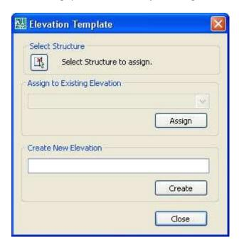
Note: If you selected a frame before the command is run, that "pre-selected" frame and its associated run would automatically be selected when this window appears. There would be no need to click on the **Select Structure** button.
