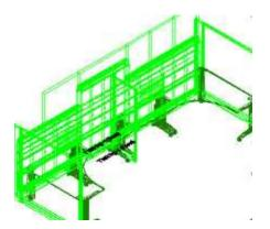
Behind the scenes, the Bind Covers command has copied all the parts in the elevation template to all of the 2D and 3D Cap standards linked to the elevation template. All the parts on the 2D and 3D Cap Standards will show up on a take-off.
